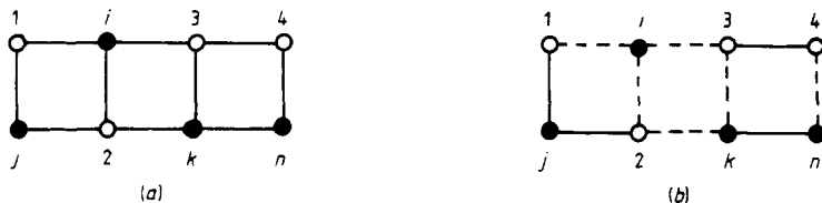
Figure 1. Example of a partial graph (b) of a graph G (a) with roots 1, 2, 3, 4 (indicated by open circles) partitioned into b' = 2 blocks: B_1 = \{1, 2\} and B_2 = \{3, 4\} . The missing edges are represented by broken lines and the non-rooted vertices by full circles.
